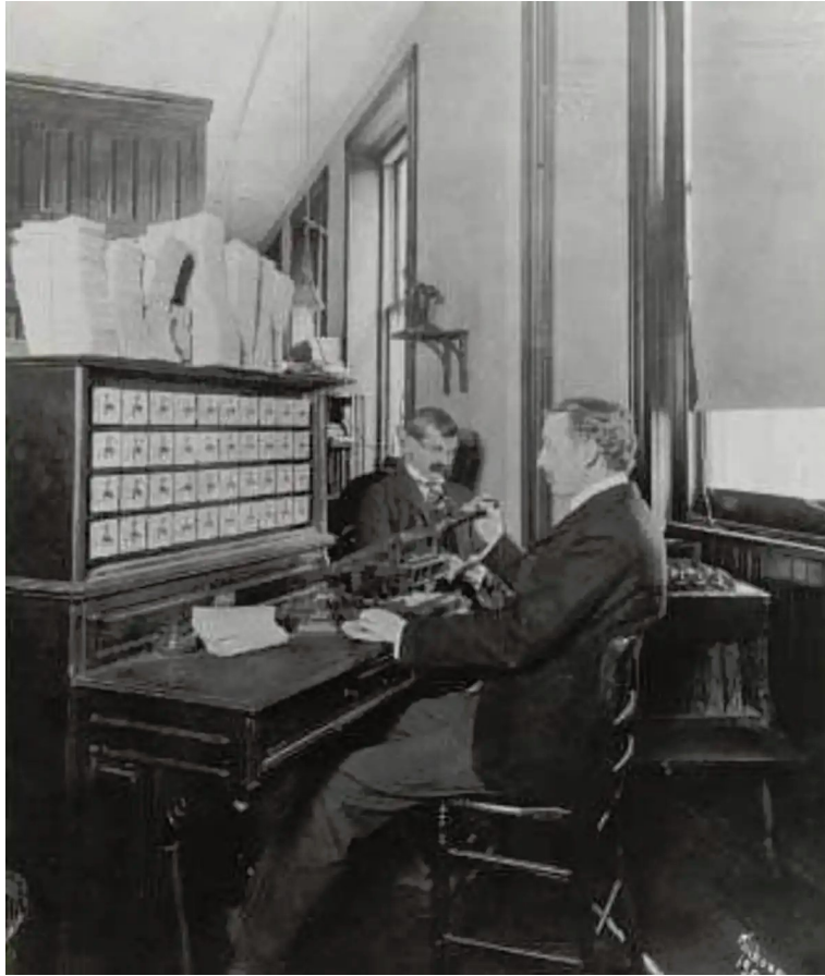
The Hollerith electric tabulating machine in use in 1902. United States Census Bureau
